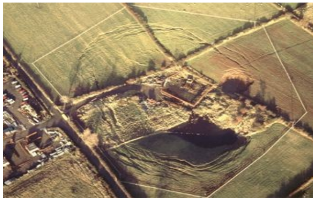
Figure 2: Wide-area subsidence and resulting new water bodies (source: Geological Survey of Ireland)
