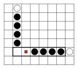
When then scanning vertically, the algorithm finds a second threat and marks it as shown at left below. The algorithm considers this case to be two threats, but in reality there is only a single threat which White can neutralize by placing a stone as shown below at right.
