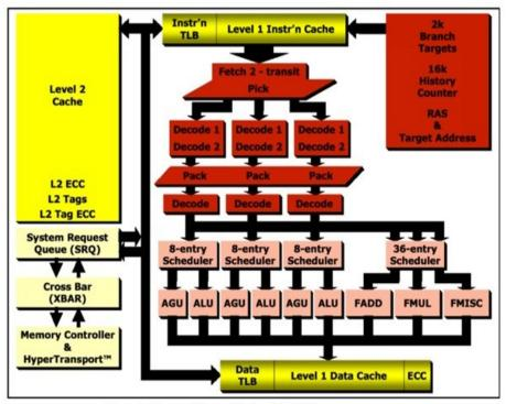
Figure 1: Hammer Microarchitectural Block Diagram
